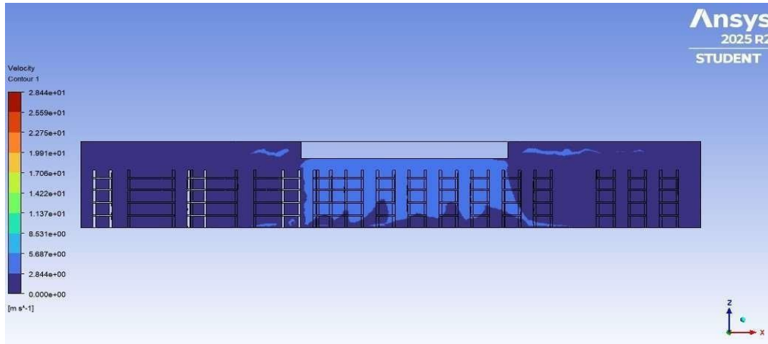
Figure 2: Velocity Contour for Central Ceiling-Mounted Evaporator Unit
