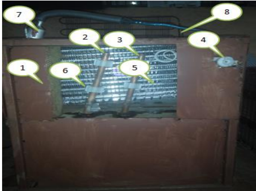
1- A.C Body, 2- Heat Pipe-1, 3- Heat Pipe-2, 4- Thermostat, 5- Evaporator coil, 6- Radial fin, 7- Accumulator, 8- Expansion valve, 9- Condenser, 10- compressor, 11- Blower.
