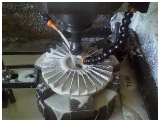
Fig. 4. Machining of heat sink model on VMC
