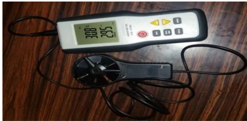
Fig. 4. Velocity measurement using anemometer
