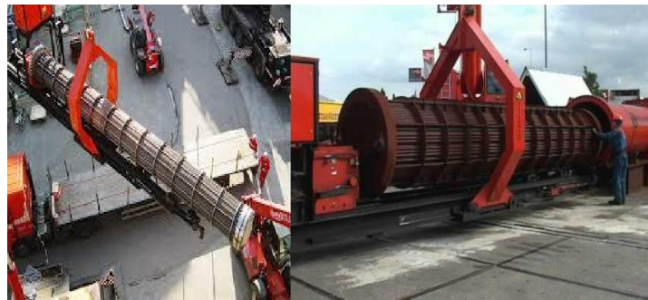
Figure 1. Manual tube bundle insert
