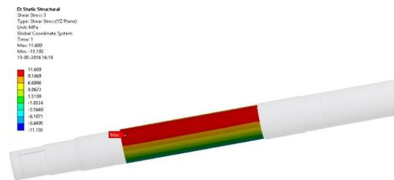
Figure 6. Maximum Stresses Induced in the shaft
