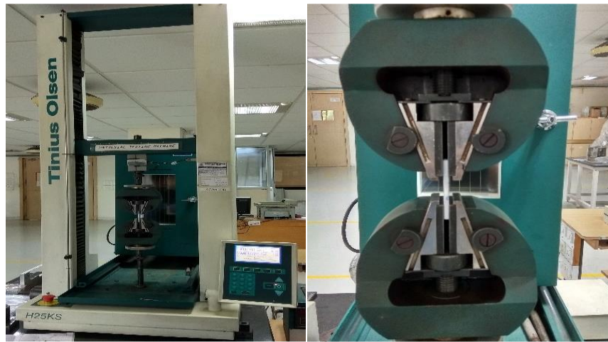
Figure 4. Tensile testing machine (Auto cluster, Pune) and sample loading on UTM
